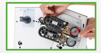
**6.** Once the belts are replaced, push down on the lower heating block to return the lever to its original position and screw the protective covers back on.
