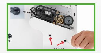
**2.** On the lower heating block, push down on the left side and simultaneously slide the lever in a downward left motion to lock the heating unit in place.
