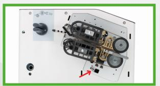
**3.** Push the lower heating block toward the right to release the tension and slide the belt away from the heating unit.
