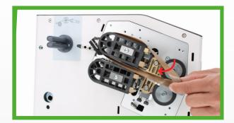
**5.** Slide the new belts onto the lower and upper heating blocks.
