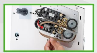
**4.** Push the upper heating block toward the right to release the tension and slide the belt away from the wheel.
