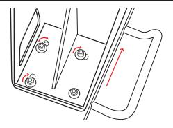
6. WITH ALL FOUR BOLTS IN PLACE, TWIST THE FILM HOLDER CLOCKWISE INTO PLACE. ONCE PROPERLY ALIGNED, TIGHTEN ALL FOUR BOLTS.
