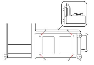
2. PLACE THE PLATFORM AND MACHINE ON ITS SIDE LINING UP THE HOLES ON THE MACHINE TO THE BOLT HOLES ON THE PLATFORM. SECURE THE MACHINE TO THE PLATFORM USING THE SCREWS WITH NO WASHERS.
