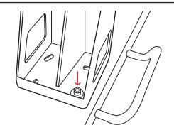
4. IN THE BOTTOM RIGHT CORNER, USE THE ALLEN WRENCH TO BOLT DOWN THE WASHER. DO NOT TIGHTEN UNTIL STEP 6.
