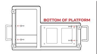
1. **INSTALL THE HANDLES ON BOTH SIDES** OF THE PLATFORM USING THE APPROPRIATE ALLEN WRENCH AND BOLTS WITH WASHERS.
