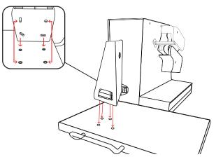
3. PLACE PLATFORM UPRIGHT. LINE UP FILM HOLDER WITH THE FOUR BOLT HOLES.
