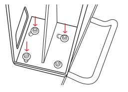
5. SCREW IN THE OTHER THREE BOLTS WITH THE WASHER USING THE ALLEN WRENCH. DO NOT TIGHTEN UNTIL STEP 6.
