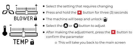
Note: Parameters cannot be set after locked. The machine will automatically lock after a period of no activity with the lock button. Adjusting parameters to the blower too high can cause film issues. If issues occur return the blower parameters to original position. Reference page 14 for troubleshooting issues.
