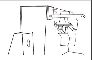
5. TAKE THE FILM ALIGNMENT BRACKET AND ALIGN THE HOLE ON THE BRACKET TO THE HOLE INDICATED IN THE EXAMPLE ABOVE. SECURE THE BRACKET WITH THE BLACK SCREW THAT IS PROVIDED IN THE SPARE PARTS BOX.
