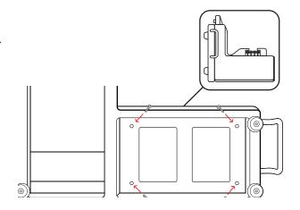
2. PLACE THE PLATFORM AND MACHINE ON ITS SIDE LINING UP THE HOLES ON THE MACHINE TO THE SCREW HOLES ON THE PLATFORM. (REFER TO THE IMAGE ABOVE FOR REFERENCE). SECURE THE MACHINE TO THE PLATFORM USING THE SCREWS THAT DO NOT HAVE WASHERS.
