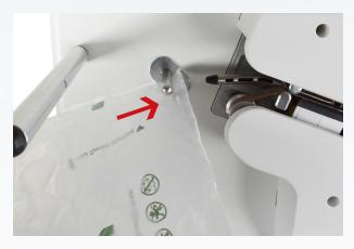
**STEP 11:**Load film onto film roller with arrows facing towards the machine. Film will go under film align rod and in-between double rods.
